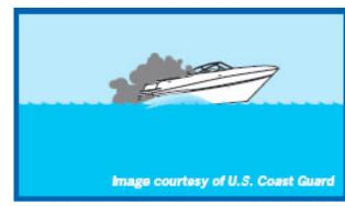
Back drafting can occur when a boat is operated at a high bow angle.
